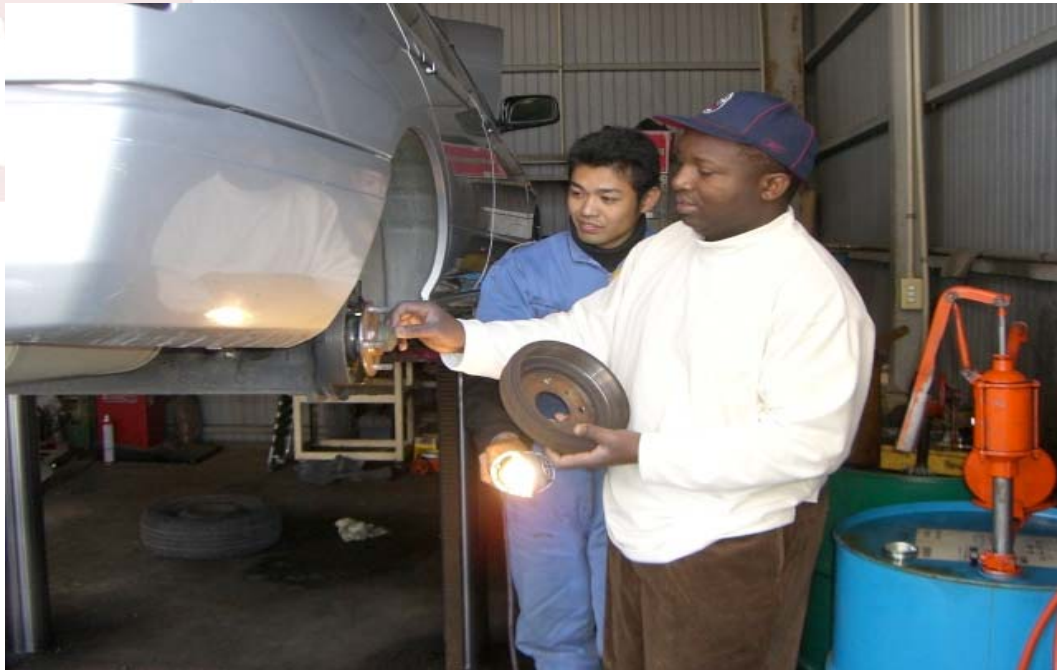
The braking system also undergoes a total overhaul. 1998 Nissan Blue-bird for Mr.Wilson C. Zimbabwe
